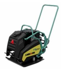
APF 20/50 DIESEL WEIGHT: 106 kg (234 lb) MAX. VIBRATING FREQUENCY: 90 Hz (5400 vpm) MAX. CENTRIFUGAL FORCE: 20 kN
